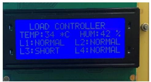
Figure 4.2 when circuit has short circuit
