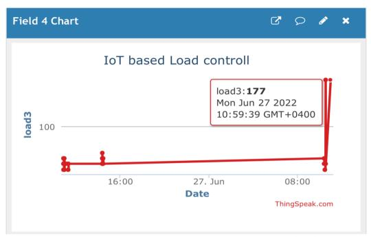
Figure 4.9 Load3 graph when occure short circuit
