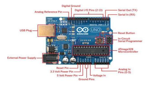
Figure 2.1 Schematic Diagram of Arduino <sup>1</sup>
