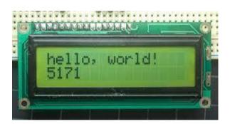
Figure 2.3 LCD display<sup>3</sup>
